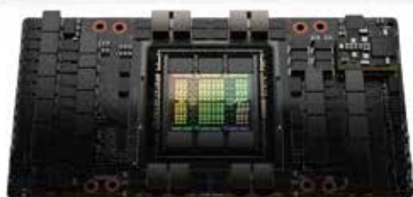
Nvidia H100 SXM5 94GB HBM2e (Hopper), 960 units in total
